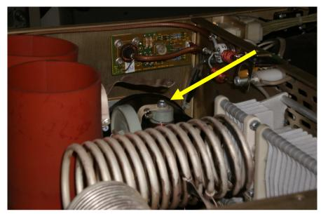
Figure 4. Remove Parasitic Suppressor Strap from Plate Choke
