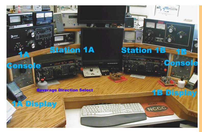
*Figure 5. K6XX SO2R Station 1 showing the antenna select system operator interface.*
