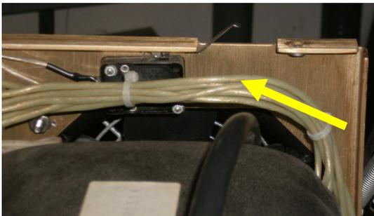
Figure 6. Rear Panel Line Interrupt Switch
