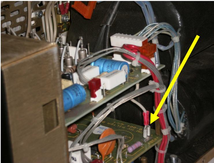
**Figure 2. Screen Supply—Connected**
