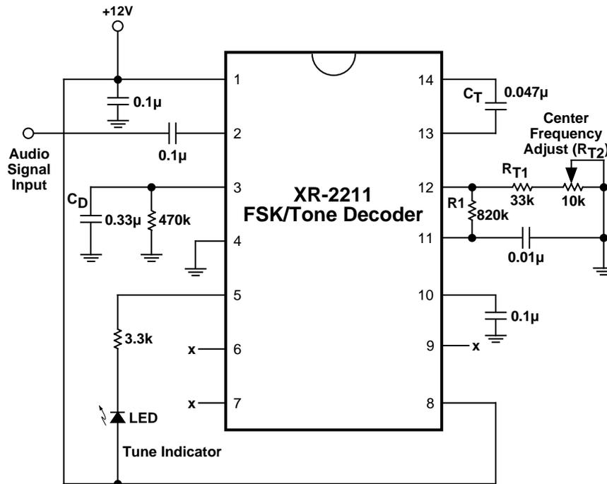
*The “Visible CW Tuning Indicator” flashes an LED when the signal is properly tuned.*
